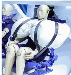
Seat Centric Restraint System (SCRS)
